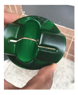
When the skimming device is removed, you can see the adhesive tape and the hardware used to capture card information from the magnetic strip.
